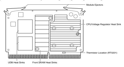
Figure 6. CPU Module Components
